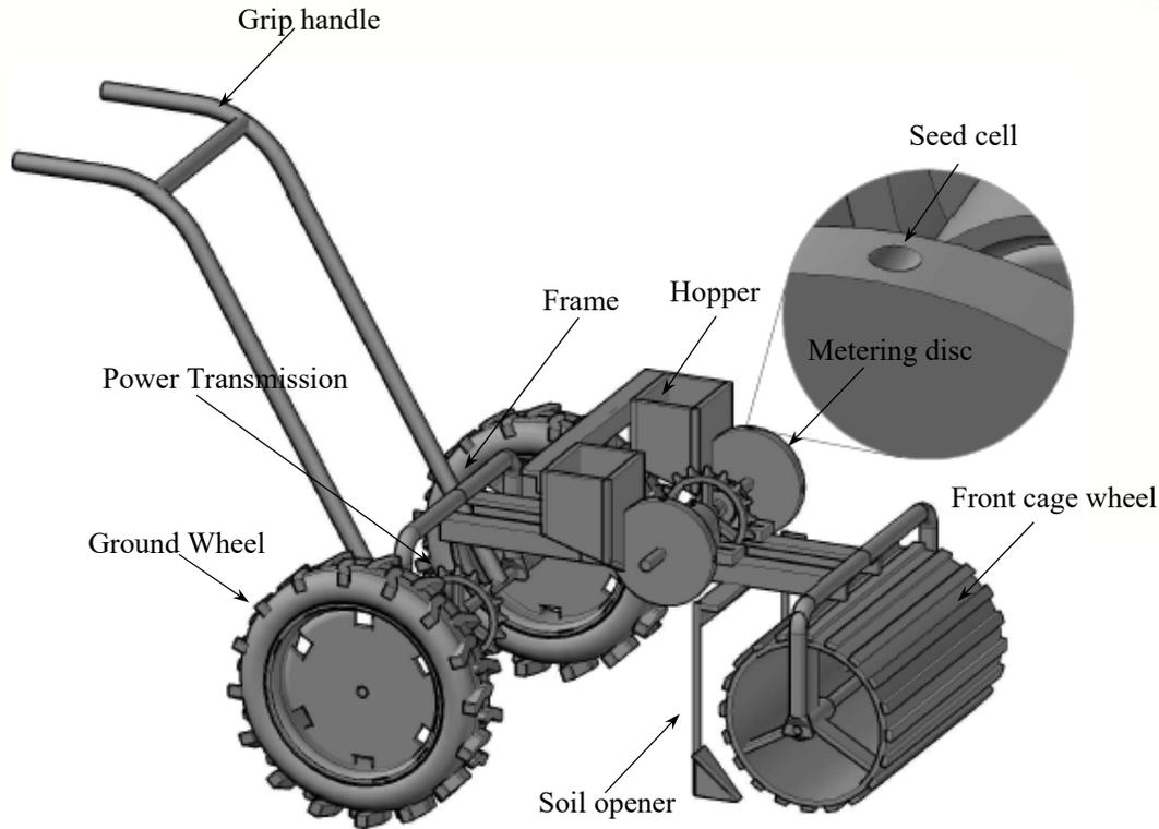
Figure 1. Isometric view of the carrot seeder
