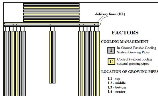
Figure 1. Experimental layout (top view of growing pipes)
